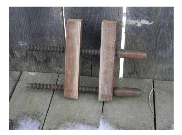
Ye old glass plate polishing vice. Well, it started out as an antique carpenter's vice and was modified for the purpose of holding a glass plate up to 8x10 in size, nice and steady, while the plate is buffed clean. These are not an essential tool for glass cleaning and actually are somewhat clumsy to work with but they do make for a good show when demonstrating the process before a group. Wow! them for only: \$85
